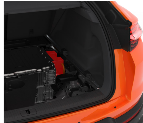
Disconnection of the 48 V vehicle electrical system for the Lamborghini Urus SE.
