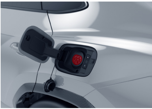
Charging socket Urus SE on the rear side panel.
