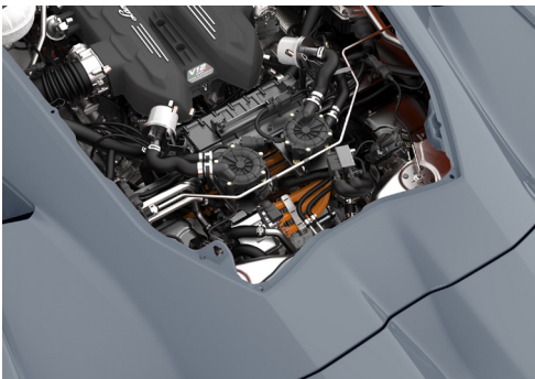
Orange high-voltage cables in the engine/motor compartment
