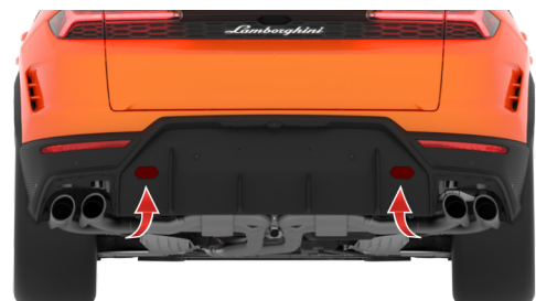
Threaded holes for the towing eyelet of Urus SE located in the front and rear bumper.
