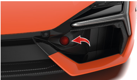
Threaded hole for the towing eyelet of Revuelto located in the front-left of the bumper.
